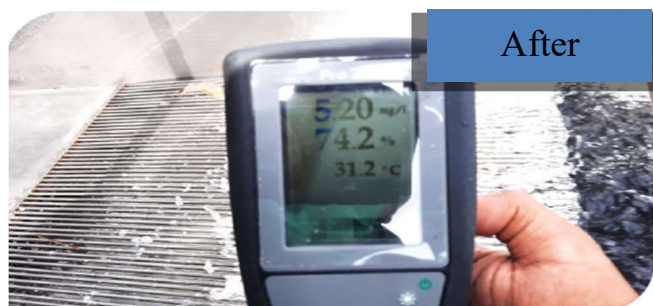
Figure 12 Measures DO Dissolve Oxygen% oxygen saturation and temperature before and after
